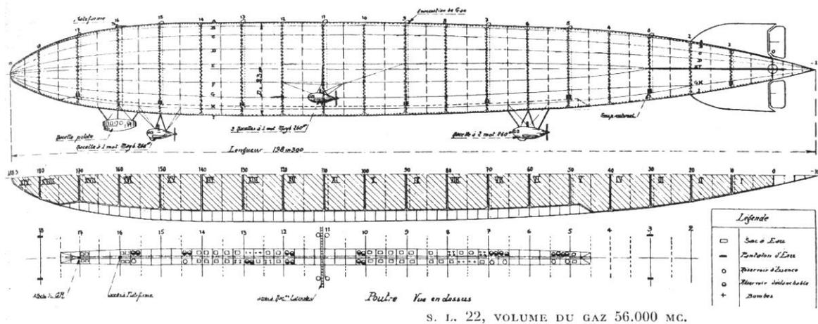
*Internal framework of an airship*
