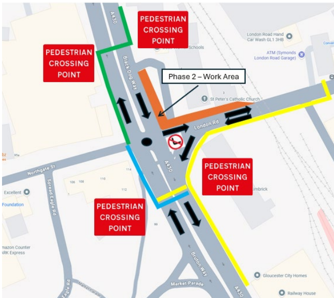
Plan B showing Phase 2 works, temporary roundabout, traffic flows and pedestrian crossings
