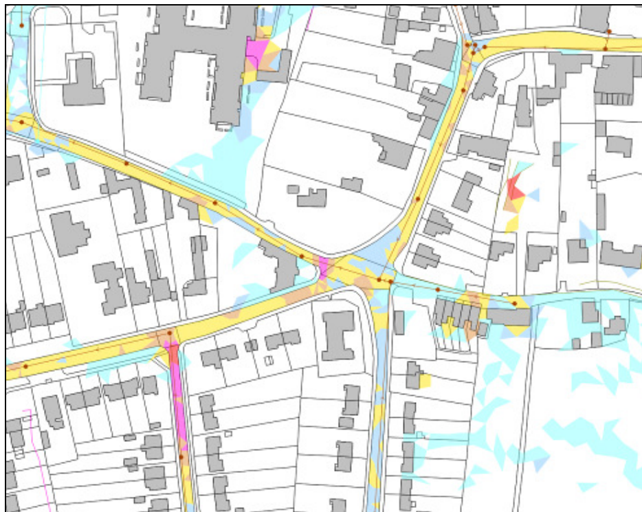
Figure 3-7 Example of how 'mesh zones' are used to replicate the flow constraints of kerblines
