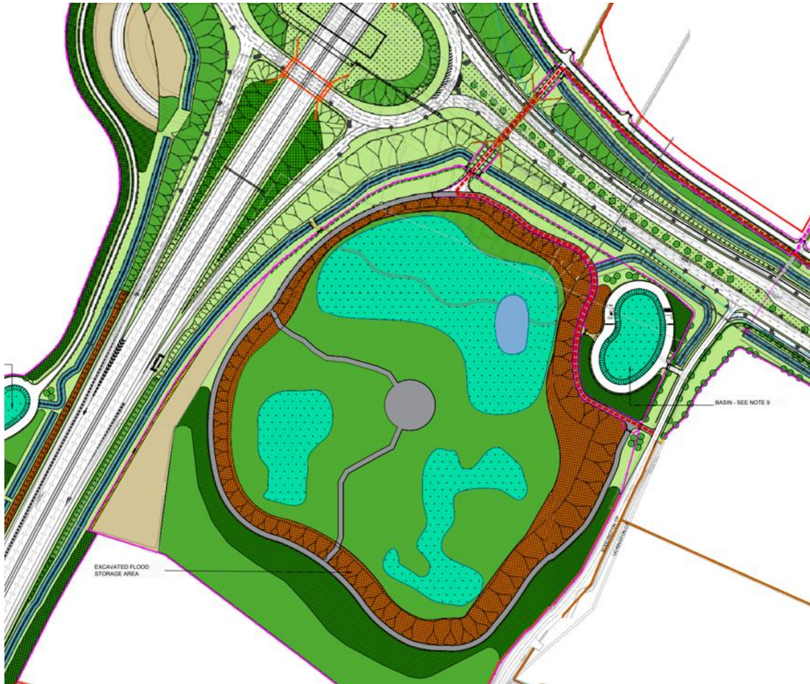
Figure 3-17 200,000m 3 reservoir in Scheme design
