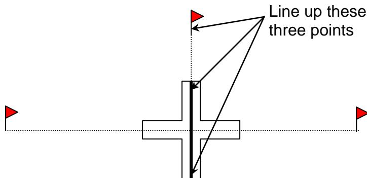
Sometimes it helps to have one of the assistants maintain one alignment while the surveyor does the other. Once the point on the baseline chain is found it should be marked with a chain peg.
