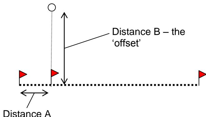
7. The surveying assistants then measure distance B (the offset), i.e. the distance from the chain out to the object. To do this, the second chain is used. One end is held at the chaining peg on the first chain and the other end taken out to the object to be surveyed. When this is done, the surveying assistants can then measure the offset in the same way.
