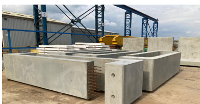
Precast concrete ground beams and parapet are currently being fabricated
