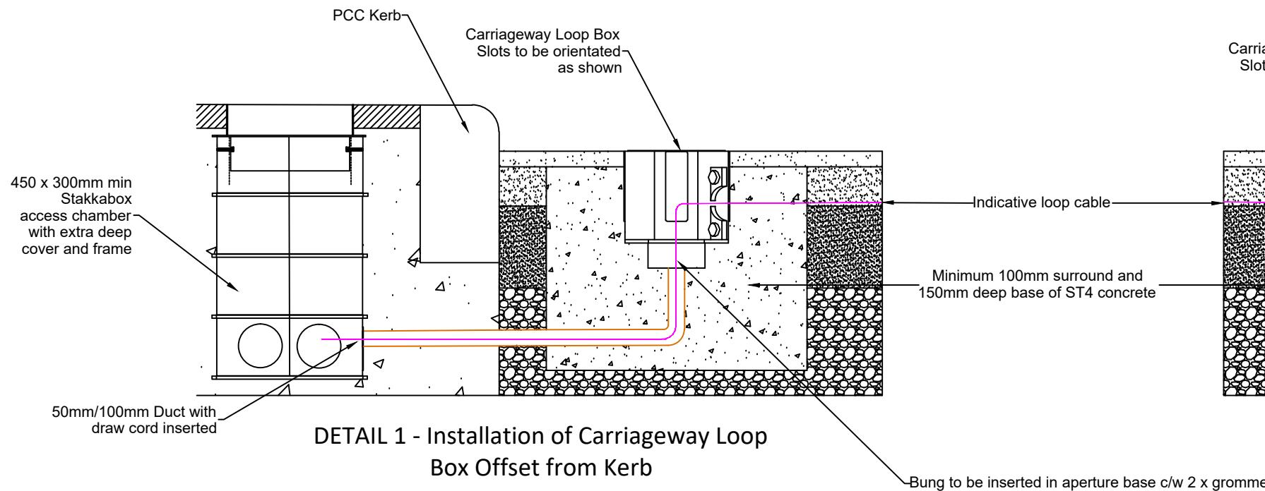
DETAIL 1 - Installation of Carriageway Loop Box Offset from Kerb
