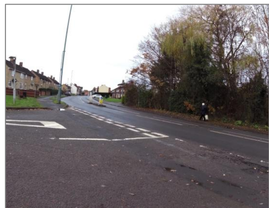
(b) End of existing shared use path at Barton Court – lack of continuity for cyclists. Junction geometry is also very wide with long crossing distance for pedestrians.
