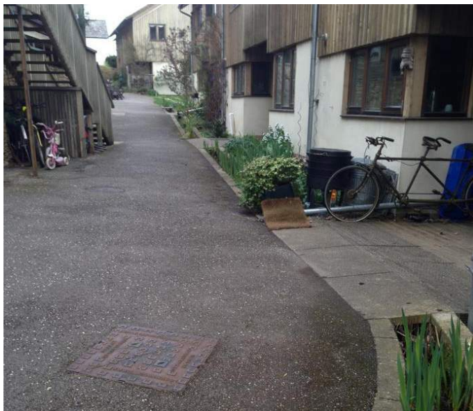
Figure 9-42 – Typical rill channel linked to downpipes
